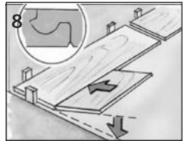
Rock and lock in half-length panel with rotating motion. Install first and second row at the same time. This will help ensure end joints are perfectly square. Planks forced down without properly engaging the tongue into the groove can result in damage.
