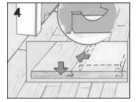
Slide panel into space horizontally and slot into profile. Use these modified planks under doorframes, radiators, cabinet fronts, etc. Use the pull bar to slide the planks where necessary.
