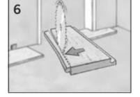
Remove the tongue on the panels that face the walls to allow room for spacers and prevent problems from spills.
