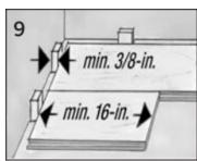
Observe 3/8" clearances for expansion and 16" minimum for smallest usable piece.
