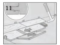
Use a 4"-6" piece to hold the tongue and groove on the same plane, limit end joint damage and ensure planks engage square. Tap end joints with multiple light taps, striking the tapping block evenly until end joints close. NOTE: Tapping too hard or striking the tapping block unevenly can result in installation-related damage or peaking.
